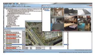
OnGuard VideoManager provides event-driven viewing and integrated alarm management. VideoManager has the scalability to grow small, simple video systems into large, sophisticated enterprise video configurations.
