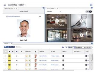
OnGuard Monitor client provides browser-based alarm management as well as live and recorded supporting video. The integrated video tilem provides a side-by-side view of text and visual event detail for reliable event monitoring and is conveniently accessible via a web browser on your desktop or mobile device.
